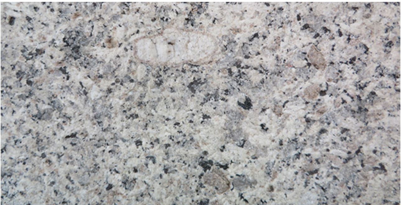
The granite used on the Submarine Memorial, note the pink feldspar and the white feldspar megacrysts with a pink rim (top centre). Field of view is ~ 20 cm.
